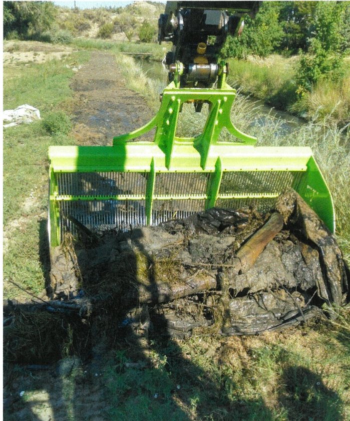
Figure 1. Aquatic Vegetation Rake
