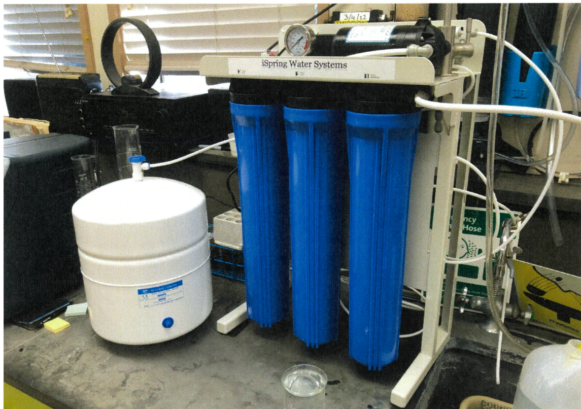
Figure 2. New RO System
